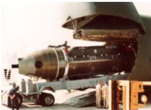
DSRV in fly-away loadout on a specially modified cargo aircraft
