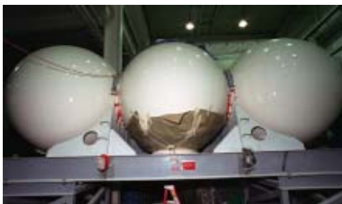
DSRV without fiberglass fairing consisted of three presurized spheres – the front is the cockpit, the back is for passengers, and the middle is for ingress and egress. Spheres can withstand the pressure of 5,000 fsw.
