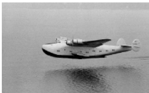
Boeing quickly removed the fin and replaced it with two at the ends of the horizontal stabilizer.
