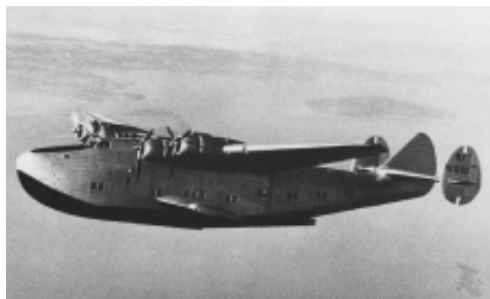
Other serious problems involved the size, shape, and location of the sponsons, or sea-wings. And, the airplane had a very bad porpoising problem on the water. Eventually, however, the location and geometry of the hull step was adjusted to resolve that problem. Here, flying on only the starboard engines.
