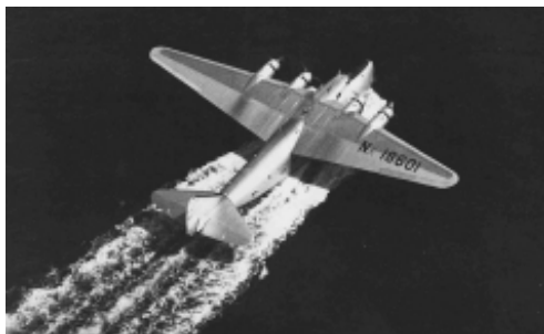
Famed Boeing Test Pilot Eddie Allen conducts a taxi test on Elliott Bay – about June 5, 1938. Notice the single (small) vertical fin.
